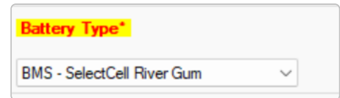
FIGURE 4.3 SP LINK Battery Type set to BMS – SelectCell River Gum.
