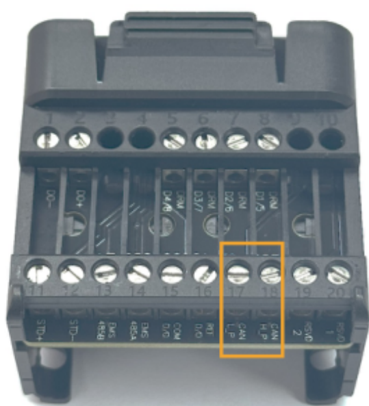
FIGURE 5.1 MHT: parallel connection on COM2 pins 17 and 18.
