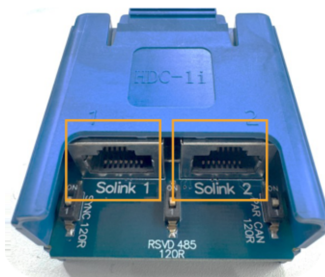
FIGURE 5.3 M2HT: Solink 1 and Solink 2 ports on COM3.
