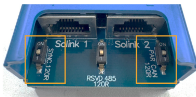
FIGURE 5.4 M2HT: SYNC 120R and PAR CAN 120R switches.
