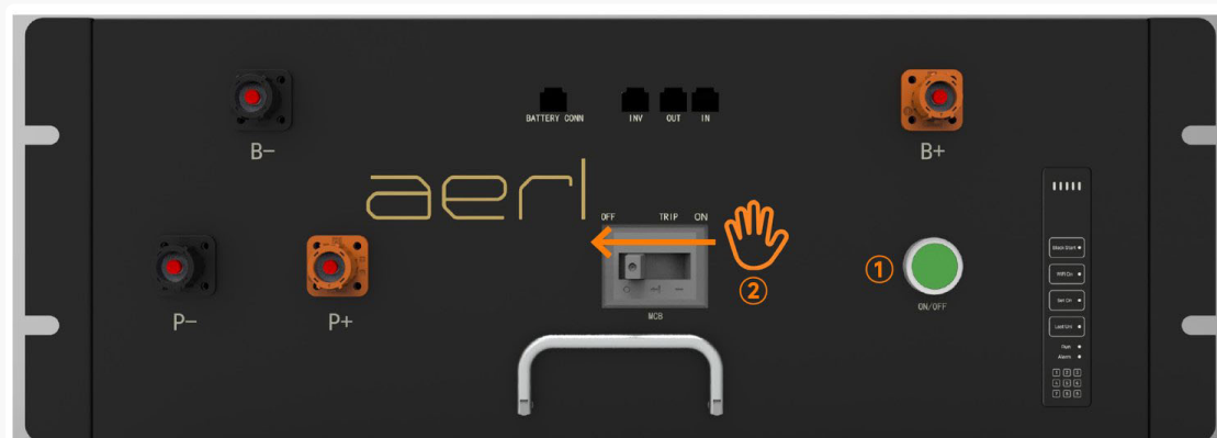
FIGURE 7.2 Shutdown sequence – hold ON/OFF ①, then confirm the MCB handle is OFF ②.
