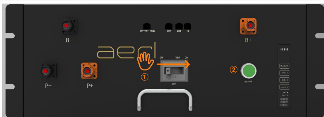
FIGURE 7.1 Startup sequence – MCB on ①, then ON/OFF ②.
